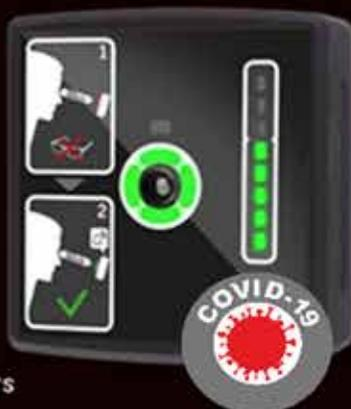
Temperature scale with 8x LED for temperature indication and display of four temperature ranges
